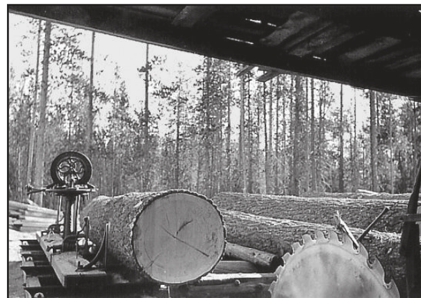
Circle saw in foreground. Log on the carriage is ready to go through the saw.
